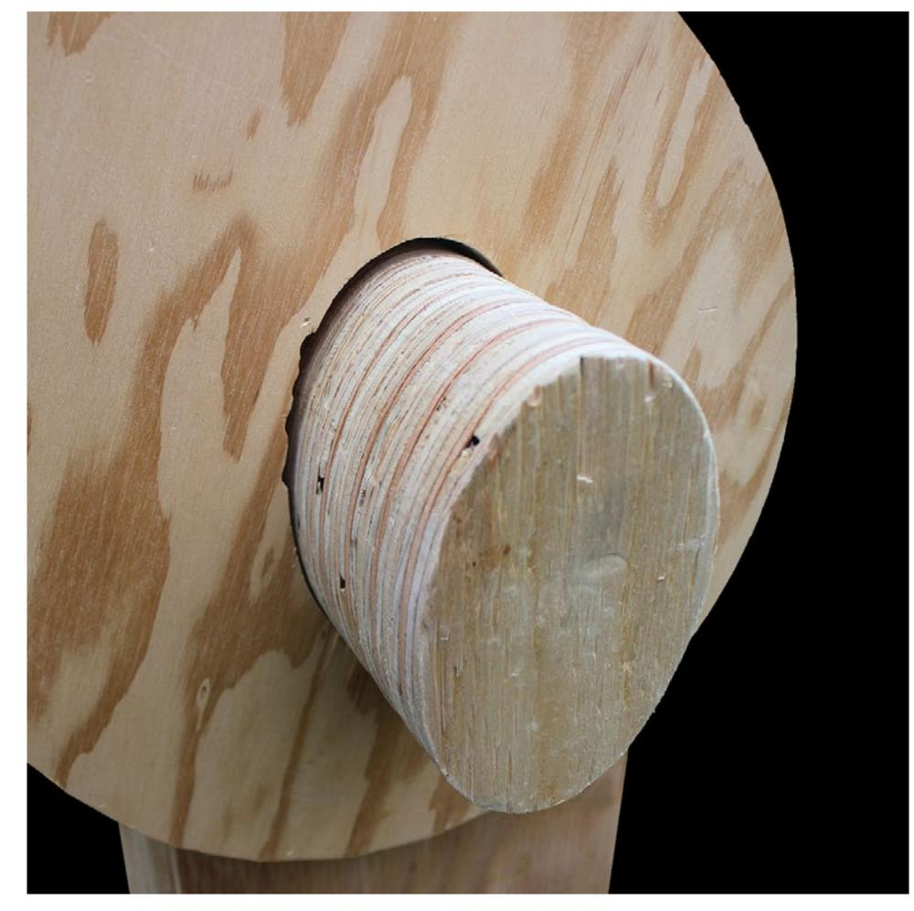
THE 1:1 MODEL is an experimental piece looking at a pin joint and the possible relationship between timber beams and columns.
