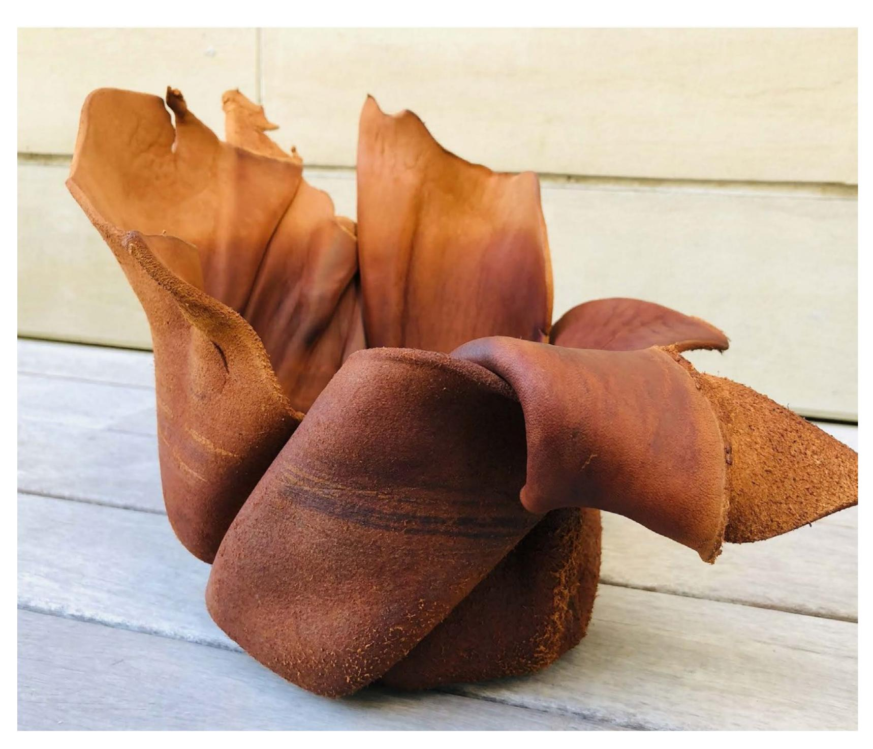
MOULDED LEATHER is leather that's been soaked in water, formed into a desired shape and can be further stiffened by oven baking. The There are varied properties of leather are in part due to the chemical and physical composition of animal skins. When leather is baked, the fibers contract and the material becomes hard and waterproof.
