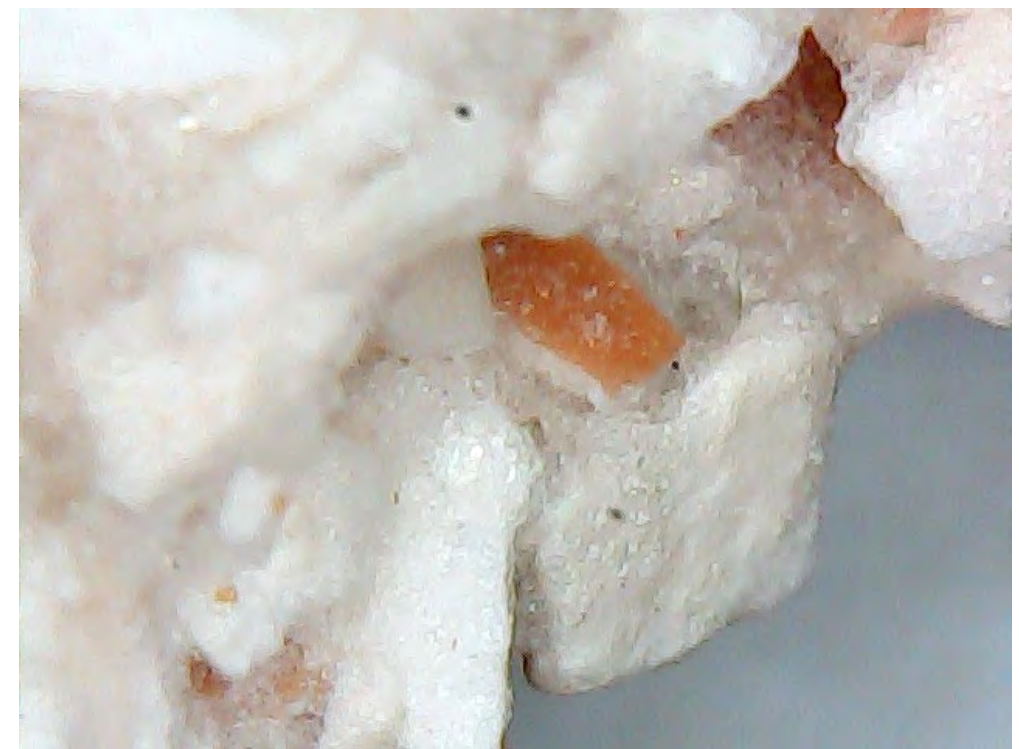
Eggshell- potato starch-shrimp based biomaterial
