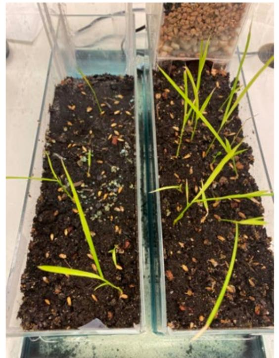
**Apparatus:** Before the main project, an apparatus was designed to demonstrate the impact of the surface runoff. Based on the record rainfall that caused the flood, which is 200 mm-hr, I calculated and found out the ideal pump to set up this condition. One side of the apparatus is mimicking the asphalt road and the other side is the pervious surface.
