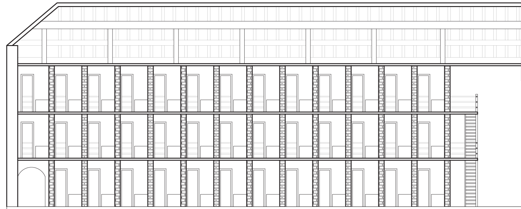
West Wing - brick masonry cells, brick exterior
