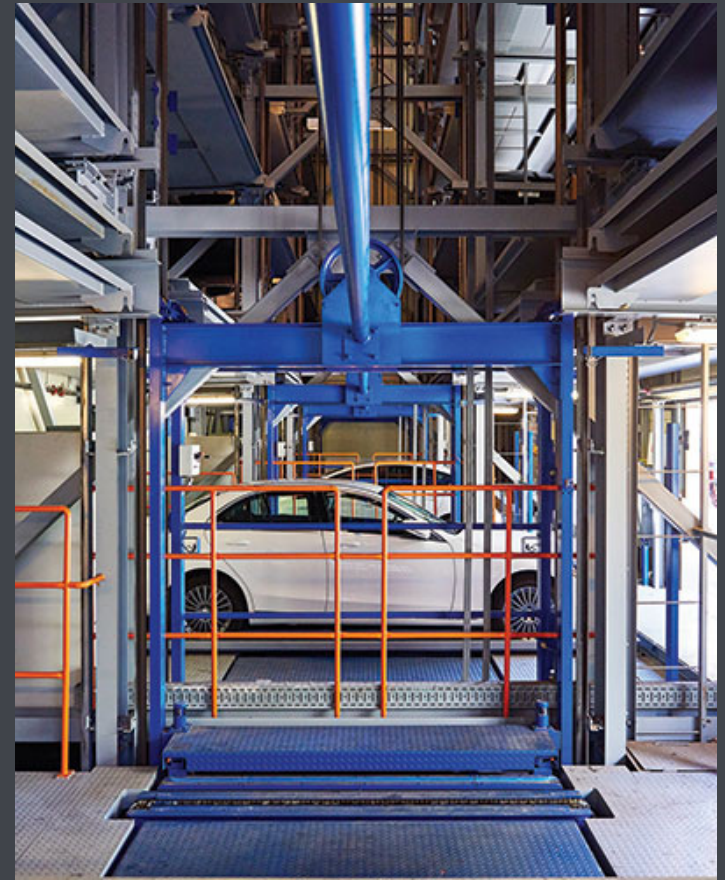
Figure 28 — The 808 Center, on the corner of Sheridan and Rycroft Streets, automated vertical parking garage that can store up to 72 vehicles (“Honolulu’s Best-Kept Secret is Out: The 808 Center”, Honolulu Magazine, April 2016)
