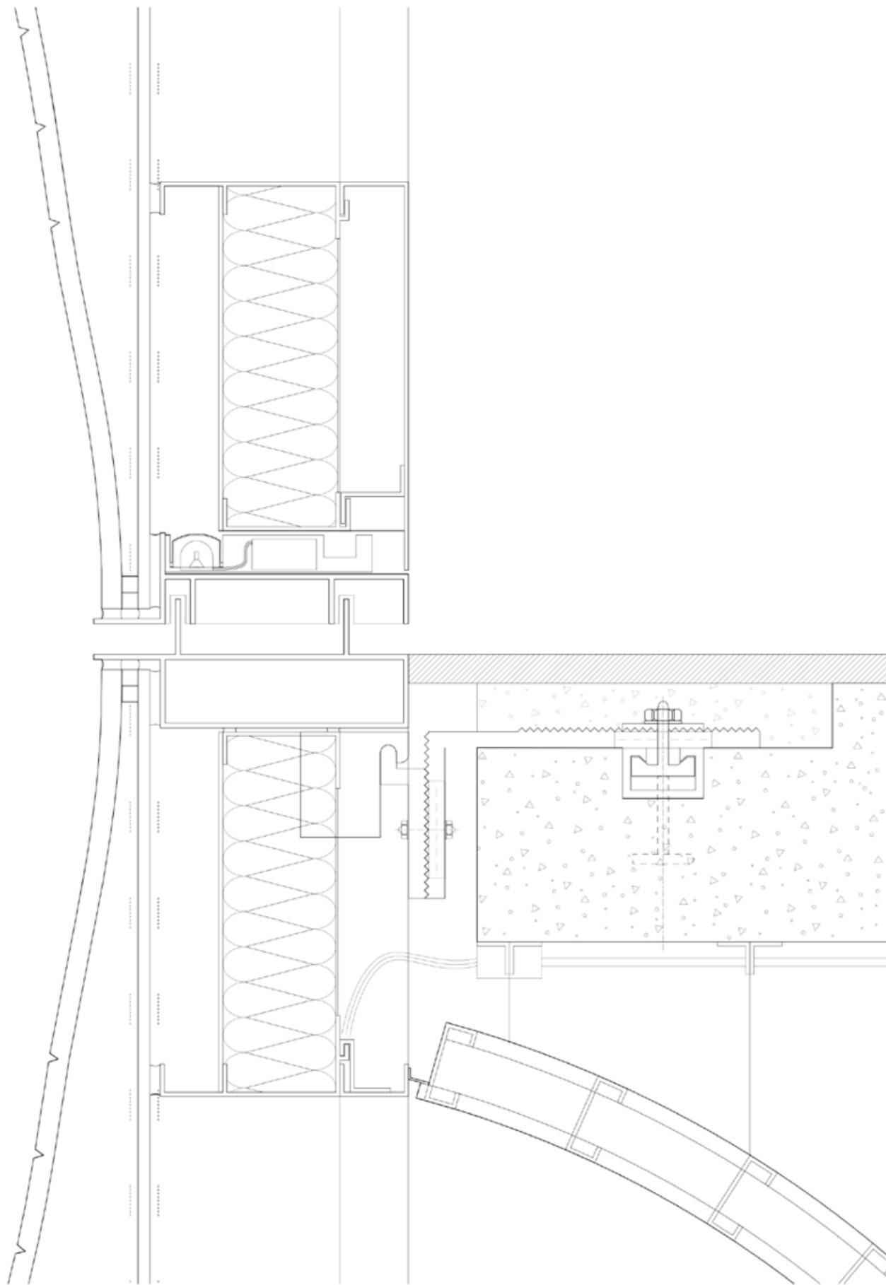
SECTION @ STACK JOINT TYP.
