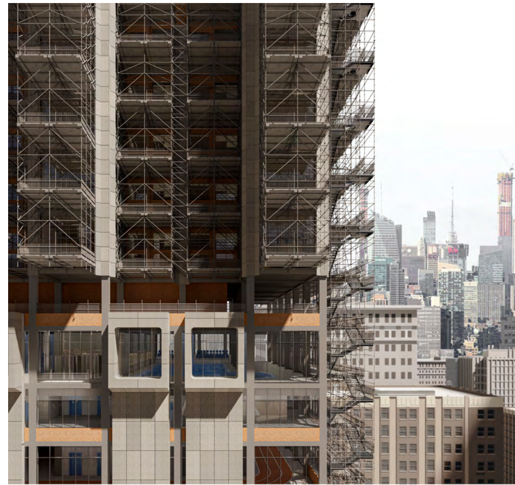
Housing and social infrastructure are gapped by mechanical trans floor. Redirect plumbing from housing to lower space.
