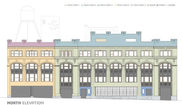
[4] Using observation and historic descriptions of the original material we determined the primary materials to include three or more different kinds of metal (the sash and doors were all originally copper, corroded to a green tint), wood, brick, four different installations of smooth white glazed terra-cotta, glass (originally wire-glazed) and granite (base). Kathleen Maloney, Seo Jun Oh, You Wu
