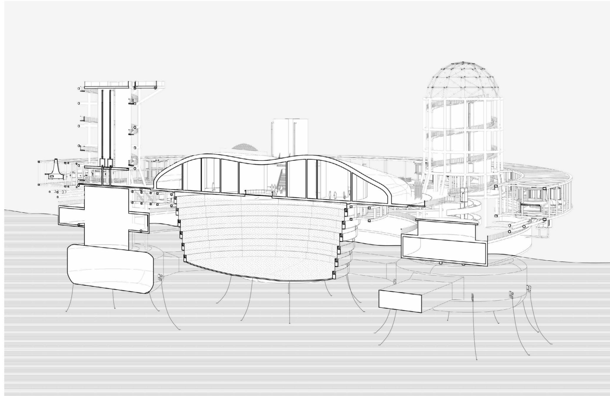
Section Perspective Cutting Through Liquid Oxygen Reservoir, and Pneumatic Oxygen Structure
