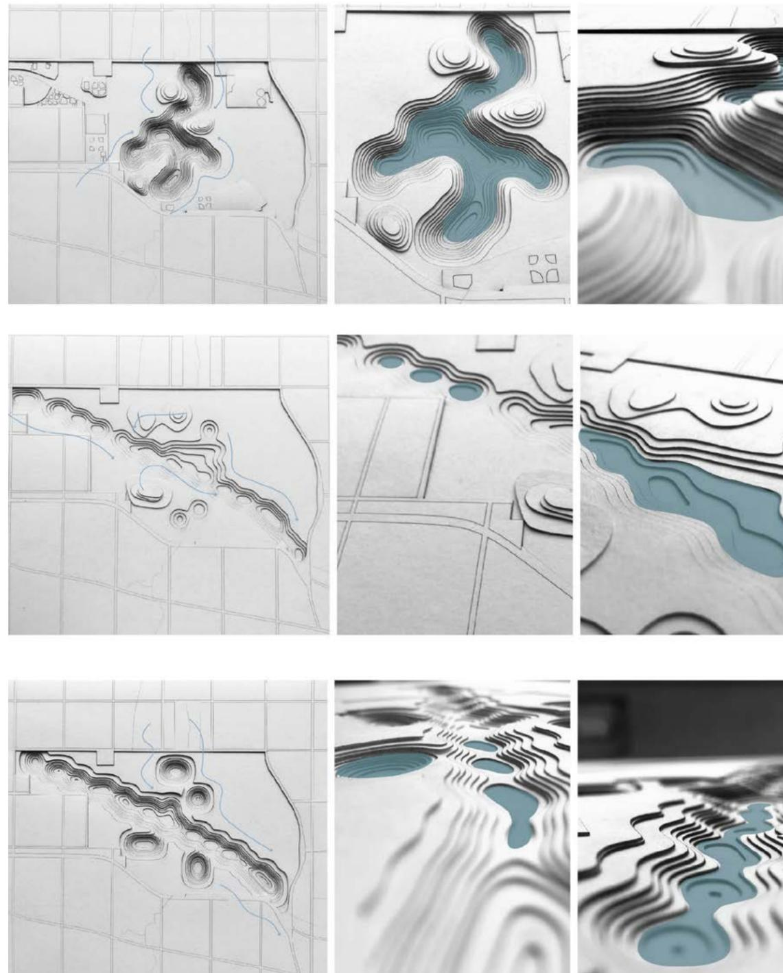
Study models of topographic cut and fill design schemes to retain water on site.
