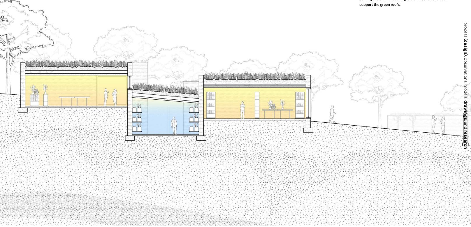
The backmost cellar is 20ft deep and stays at the average year-round temperature of 50-60F. Soil walls are excavated and retained with a wire mesh system. They are capped with rammed earth walls. Steel girders with decking sit on top of them to support the green roofs.
