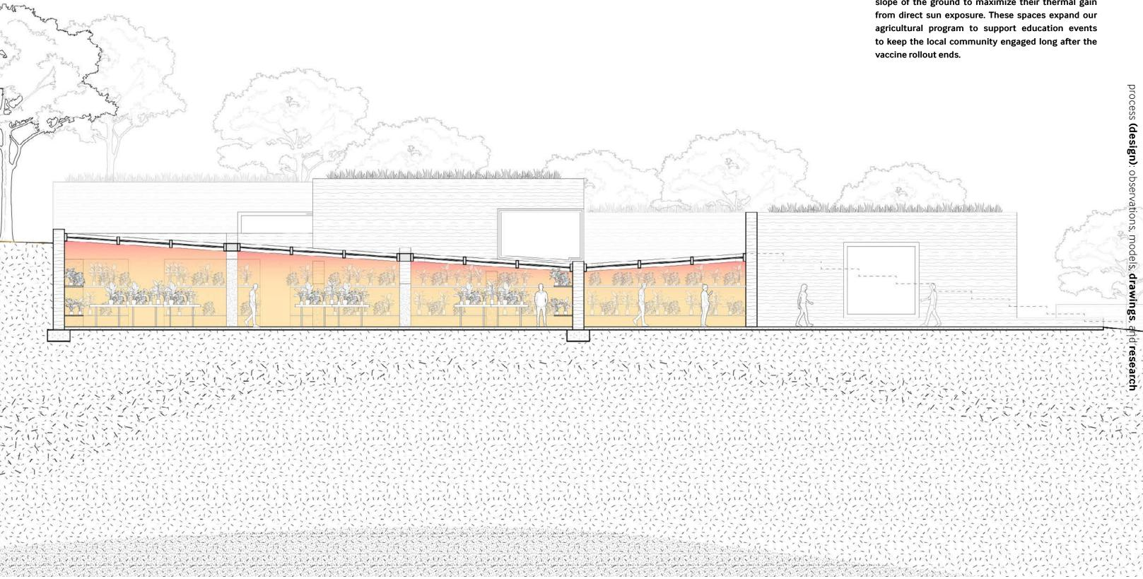
The greenhouse spaces are located along the southern end of the site and have clear roofs that meet the slope of the ground to maximize their thermal gain
