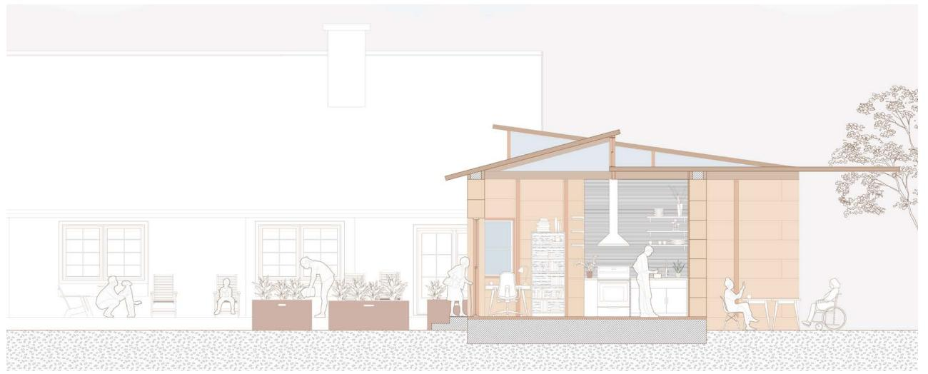
The density of the straw walls provide thermal efficiency to create comfortable domestic spaces, and utilize passive design standards to reduce energy demand.
