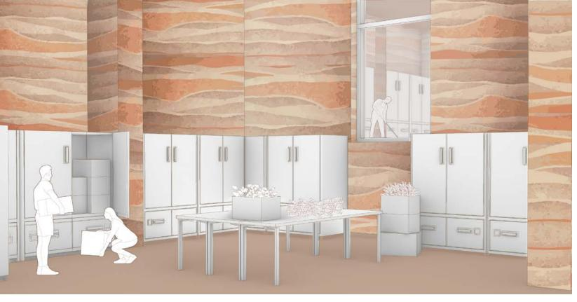
In the distant future, the site expands below ground to utilize the earth's insulation properties to store agriculture. Using a mixture of passive and mechanical interventions, varying temperatures throughout the underground cellars create hot-dry to very cold-moist conditions depending on the crop.
