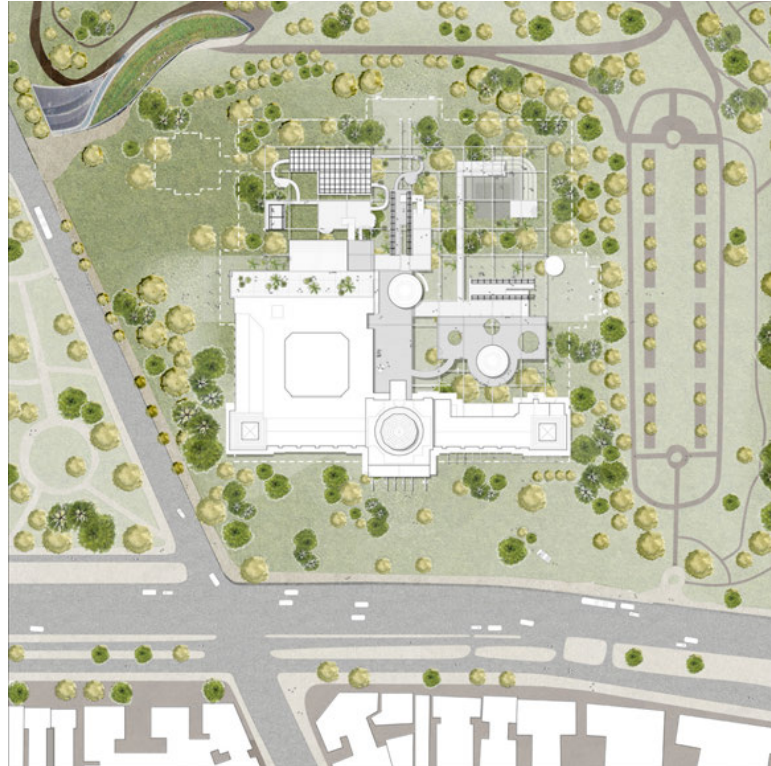
Proposed roof plan; series of platforms, walkways, stairs and ramps echo the multiple domes proposed for the unbuilt building, and structural form of the original grid plan
