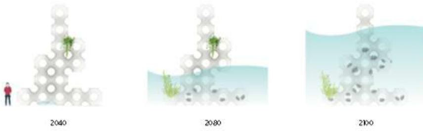
Reef balls are structures made of concrete, silt and shells. Their porous nature that mimics reef structures provides a habitat for oysters and other aquatic plant and fish species. The modular and condensed versions made of recycled glass and compacted sand can be arranged and aggregated in such a way to provide a column-like support structure.
