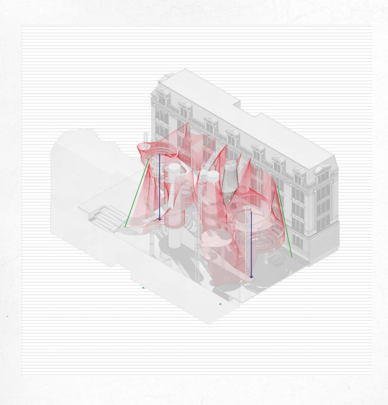
Structural Diagram showing compression and tensile forces
