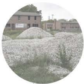
Material- Tabby Concrete Oyster Shell Collection Station
