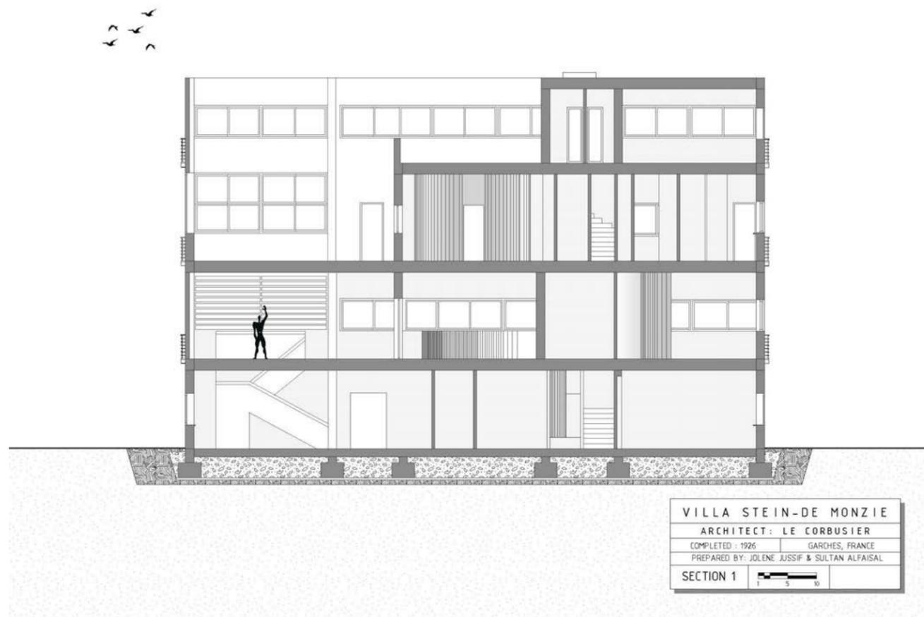
*This section displayed the conventional stacked section and carved out terrace. This section displays the ribbon windows that wrap the building.*
