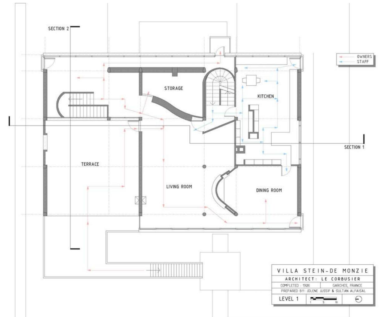
Level 1 is the owner's living quarters and can be entered directly from the ground by the terrace. This floor encompasses their living room, terrace, kitchen, and dining room. This plan displays the many configurations of a free plan.
