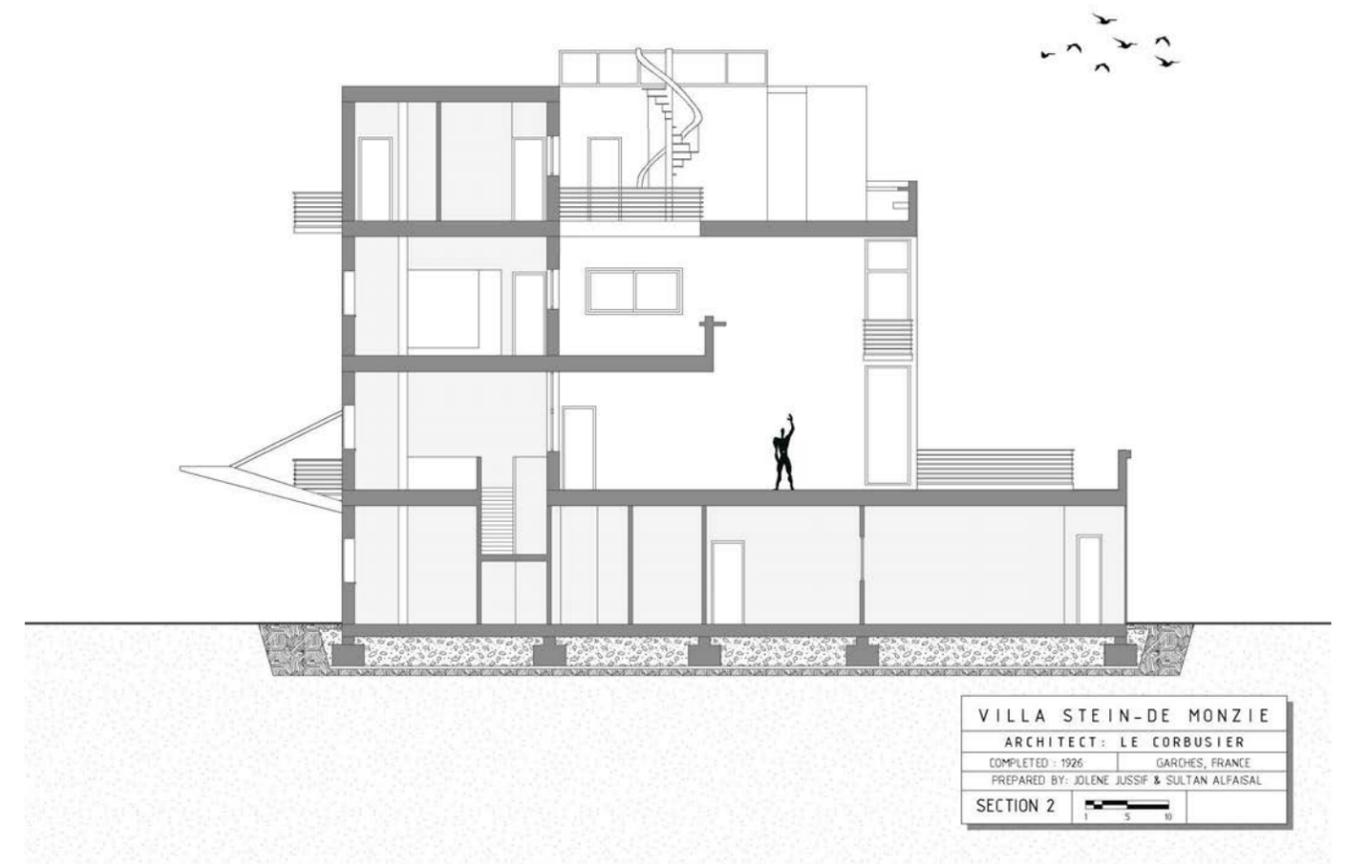
*This section displays the stepping form of the building and the detail of the handrails. The stepped facade of the building is the back and one would enter under the overhang.*
