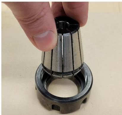
After finding the correct collet for your endmill, place the nut face down on a flat surface and press the empty collet straight down into the nut until it locks into place. It's important for the collet to be mounted straight into the nut and to not be crooked at all.
