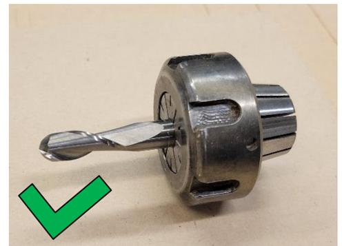
**NOTE:** Always make sure that your endmill is long enough to reach down past any vertical features of your mill file. The longer your endmill, the greater the risk that it can snap. Always try to use the shortest, thickest endmill that will work with the geometry you are trying to create. You may use this same process to install a drill bit on the mill for drilling holes, however you should never use a drill bit as an endmill or an endmill as a drill bit.
