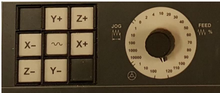
Move the center of the tip of your endmill to the point corresponding to your Rhino origin and press the **USER** (F5) button. Then press **LOAD ZERO OFFSETS** (F2), then press **LOAD G55**, then in order press **X G55**, **Y G55**, **Z G55**. Each of the XYZ tabs should say that the current origin is **LOADED**. Once all three are set, press **EXIT** (F7) three times to return to the **JOG** menu.
