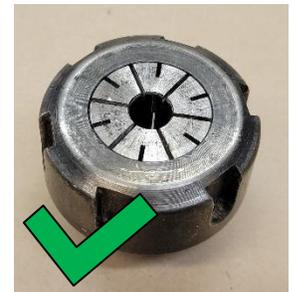
The collet should only compress on the shank, the smooth end, of your endmill. It should never cover any part of the flute, the cutting edge, of your endmill. Make sure the collet is gripping on to at least ~0.75" of the shank.
