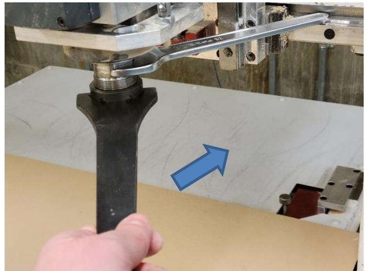
**NOTE:** When your file is finished running don't forget to take your endmill out of the machine. Go to the Jog menu and hit the tool change button. To take your endmill out, simply change the orientation of the wrenches. The Black wrench should be placed on the rail up against the gantry and then push the silver wrench to the right to loosen the nut.
