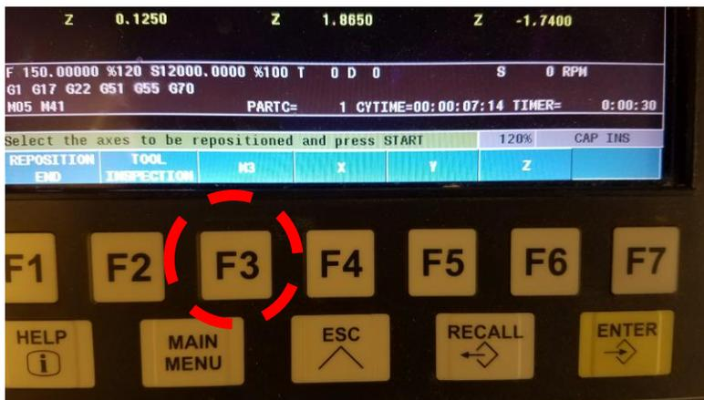
Repeat this process to reposition the toolhead by pressing **F3** to select axis you would like to move and then pressing the **green cycle start button**. Always make sure to reposition the z axis last.
