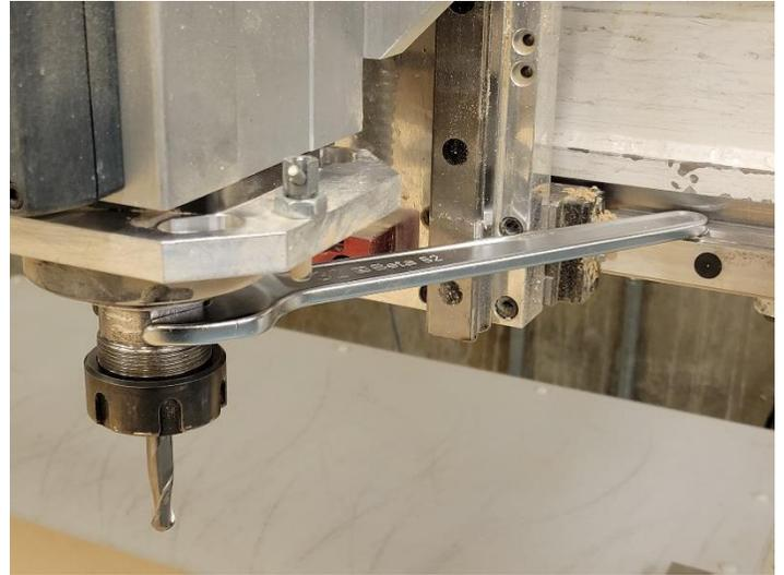
Then slide the teeth of the black wrench up into the notches on the sides of the nut. Once the two wrenches are in place, push the black wrench to the right to tighten the nut. One quarter turn past finger tight should be enough. You should also avoid over tightening the nut on to the spindle.
