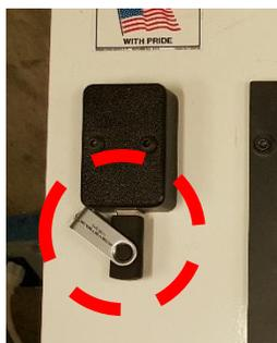
Plug your USB drive into the port on the top-left of the control panel.
