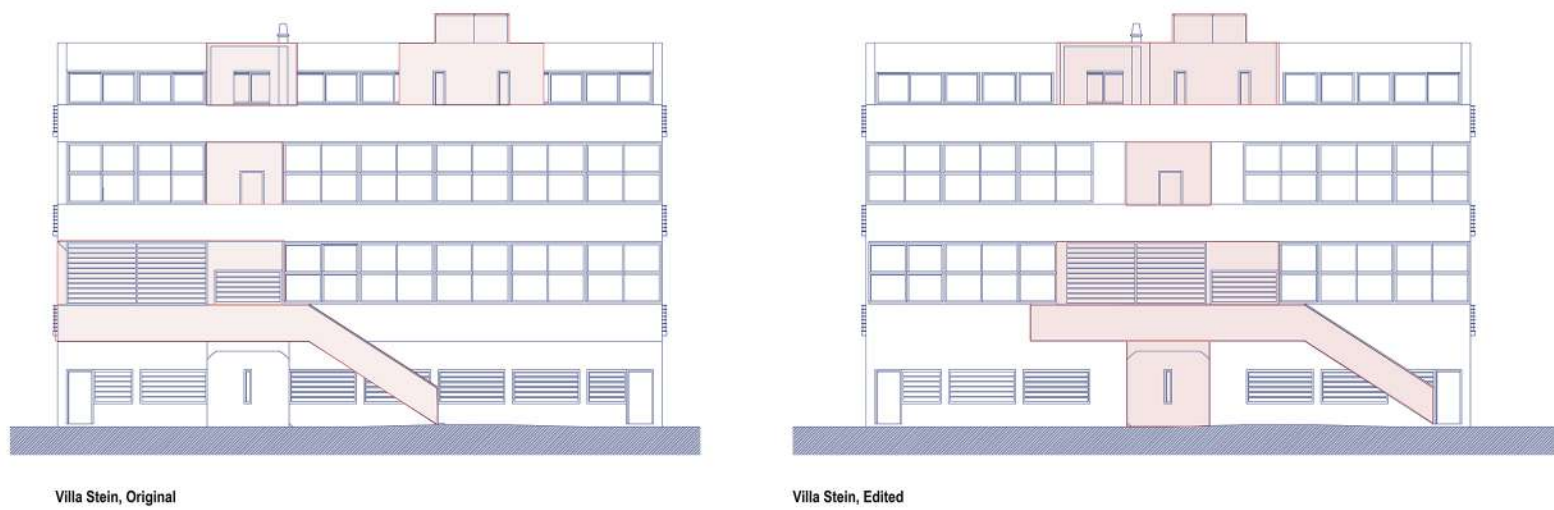
Figure 10. Front elevation of Villa Stein modified by the movement of terrace, pavilion and stairs, to the center and by breaking up the gashes of windows into two parts
