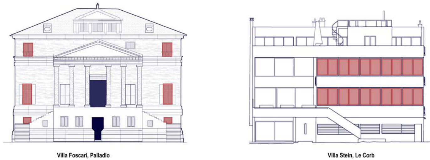
Figure 4. Placement of fenestrations on both the elevations.
