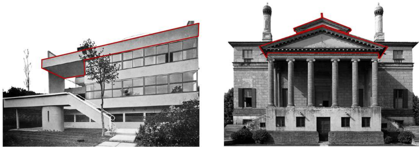
Figure 7. Additive and subtractive nature roof forms.
