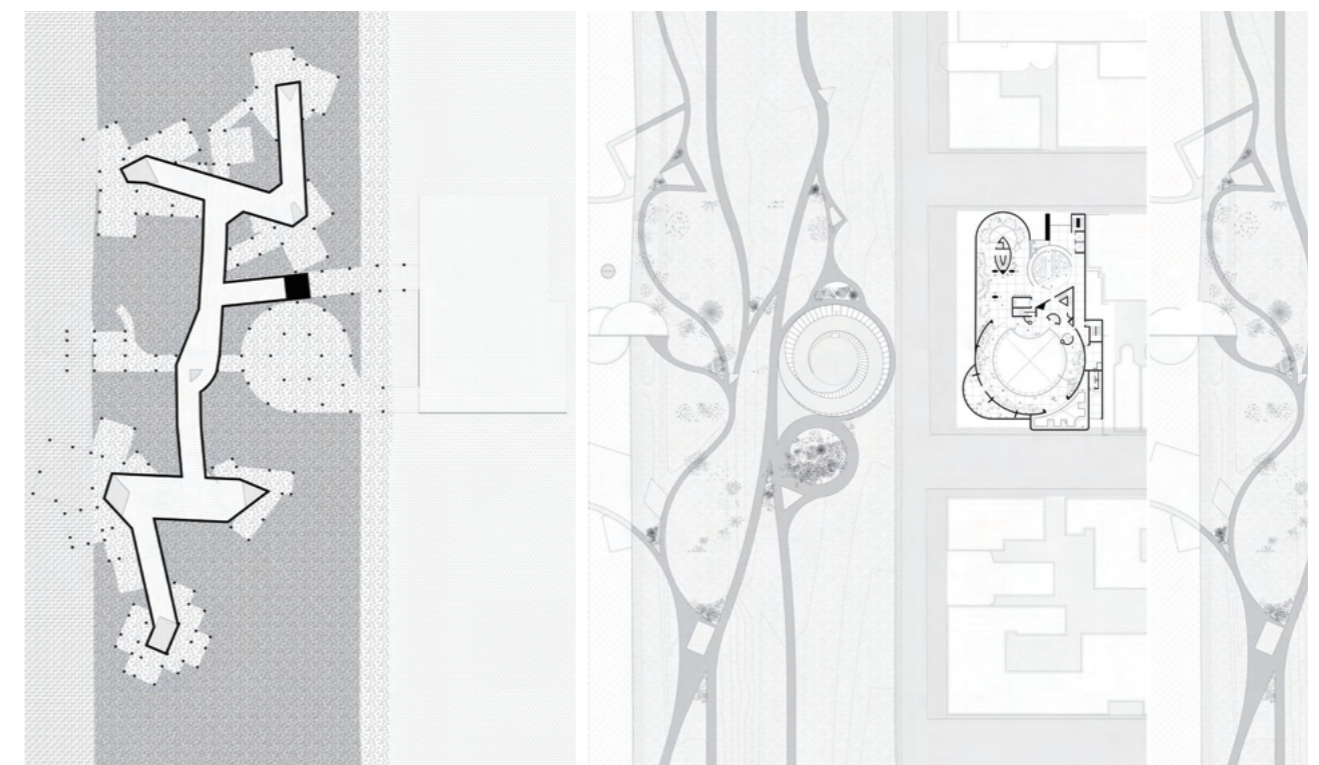
BOH Level Plan | Curators and artists are able to load material and art via wide 20 ft corridors and reach the gallery levels via a loading lift that takes the shape of the central courtyard. 4th Level Plan | The act of taking over the original building is done with wonky, customized furniture. Now, instead of being a machine for collection, it has become a laboratory for art conservation, education, and development.
