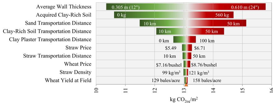
Fig. 12. Sensitivity analysis of the global climate change impacts of cob production, ranked by the input effect on output mean.
