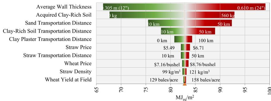
Fig. 11. Sensitivity analysis of the energy demand of cob production, ranked by the input effect on output mean.
