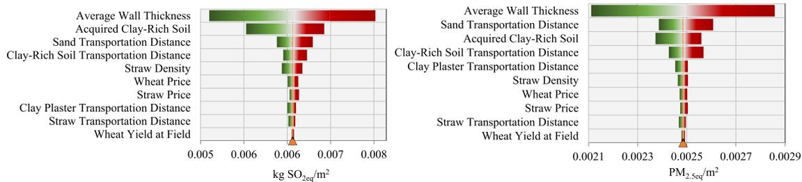
Fig. 13. Sensitivity analysis results of the air acidification (left) and HH air particulate (right) impacts of cob production, ranked by the input effect on output mean.
