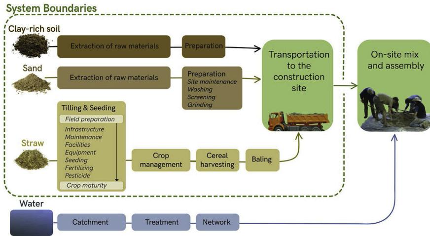
Fig. 5. The system boundaries and processes incorporated in the developed cob LCI.
