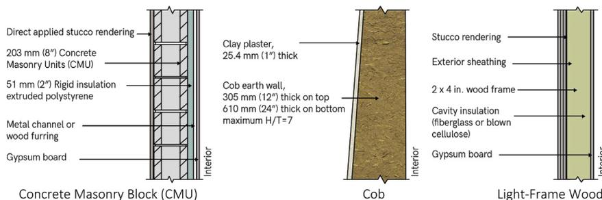
Fig. 6. Section drawings of the assessed wall systems.
