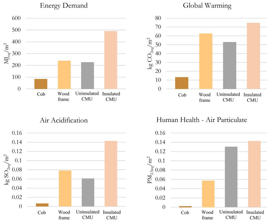
Fig. 10. Environmental embodied impacts comparison among the different wall systems.
