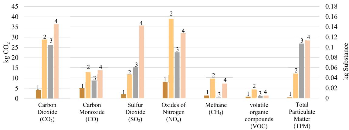
Fig. 8. LCI air emissions for each of the assessed wall systems: (1) cob, (2) wood frame, (3) uninsulated CMU, and 4) CMU with internal rigid insulation.
