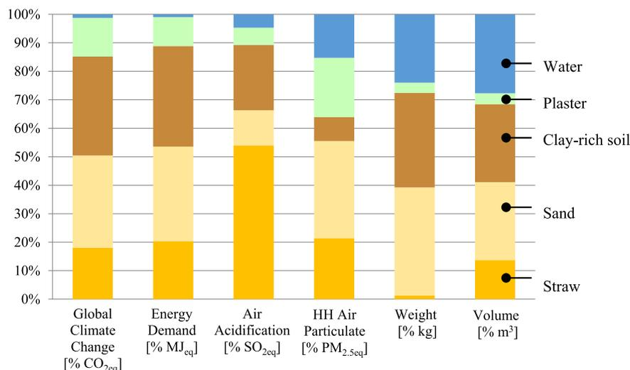
**Fig. 7.** Distribution of global climate change, energy demand, air acidification, and air particulate impacts, as well as the weight and volume for each constituent component of the cob mixture.
