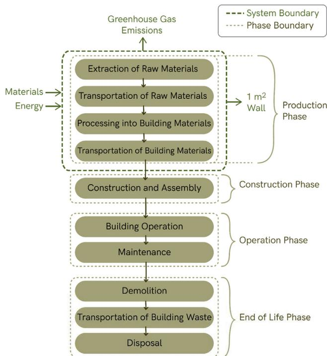
Fig. 4. The system boundaries of the proposed study, which includes the production phase from cradle to construction site.
