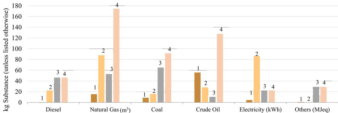
Fig. 9. LCI energy and fuels demand for each of the assessed wall systems: (1) cob, (2) wood frame, (3) uninsulated CMU, and 4) CMU with internal rigid insulation.
