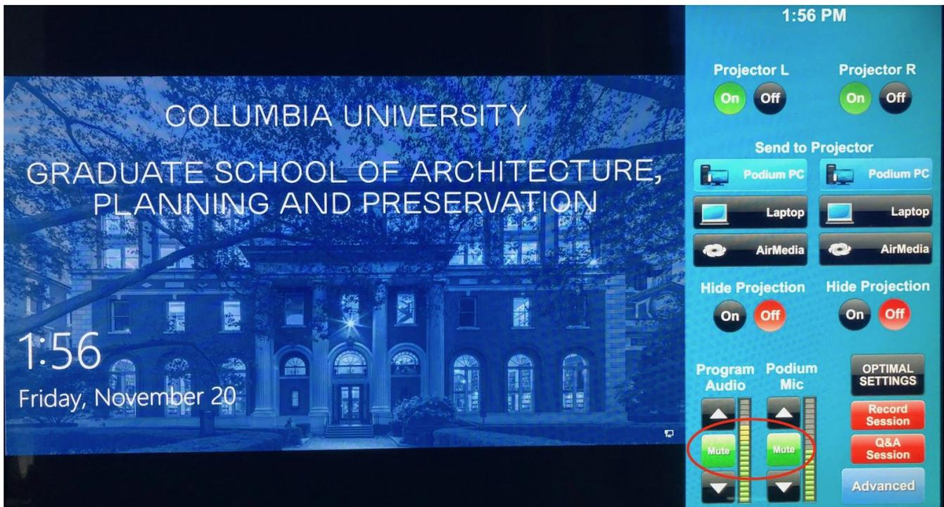
**ADJUSTING VOLUME:** There is a green bar with arrows to adjust up or down. If you do not see green on the bar, tap it at the top several times until the green scale shows up. If there is still no sound, or not enough sound, check the volume settings of the computer you are using. Additionally, if you are playing sound off a given program (Quicktime Player, Powerpoint, etc.), check the sound settings within that program.
