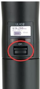
To turn on the wireless mics you'll need to switch to the "on" position. Always make sure the batteries are fully charged. Charge if needed. Keep the wireless mic off until in use to preserve battery and to prevent feedback. The battery lasts up to two hours. Audio levels can be adjusted by speaking closer or further from the mic or raising or lowering one's voice. They are set for optimal.
