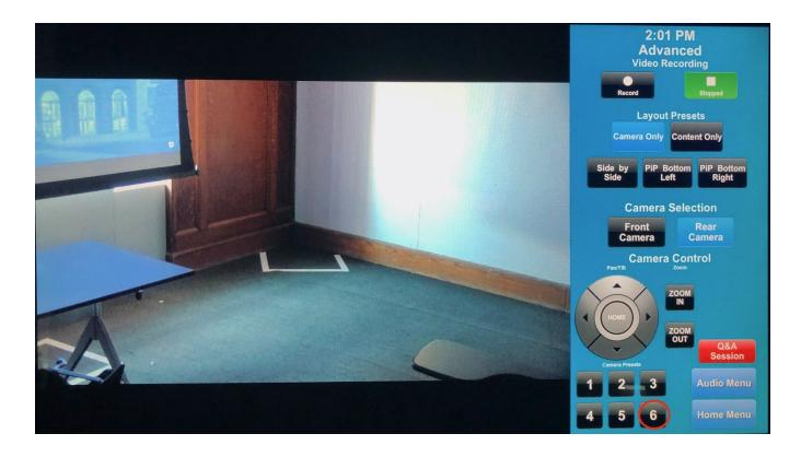
→ Set up a single camera shot that includes podium, table, and projection screen as below with Preset 4:
