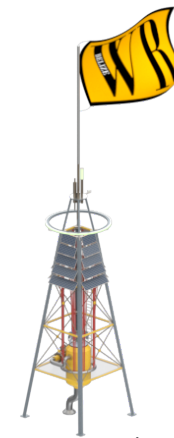
Monitoring Tower (Land) Collects water samples from the watersheds
