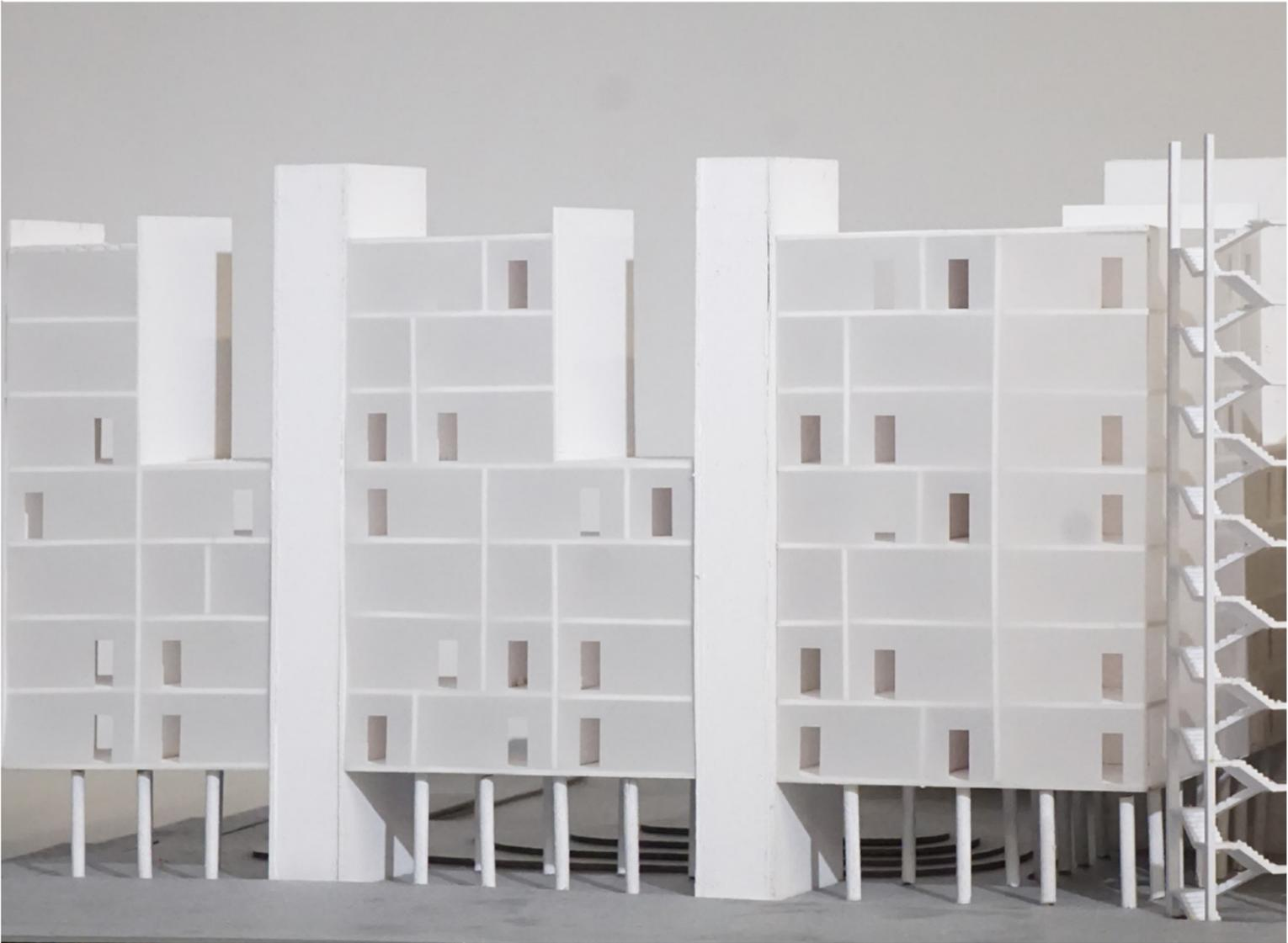
◀ Unit mix diagrams. Units are distributed to create a mix of incomes on every floor. Duplex 1BR & 2BR units are nested to relieve the need for a corridor on every third level, letting more light and air into the building. ¶ ▲ 1/16" study model, exterior circulation removed. The exposed pattern of entry doors hints at the duplex dependent unit mix.
