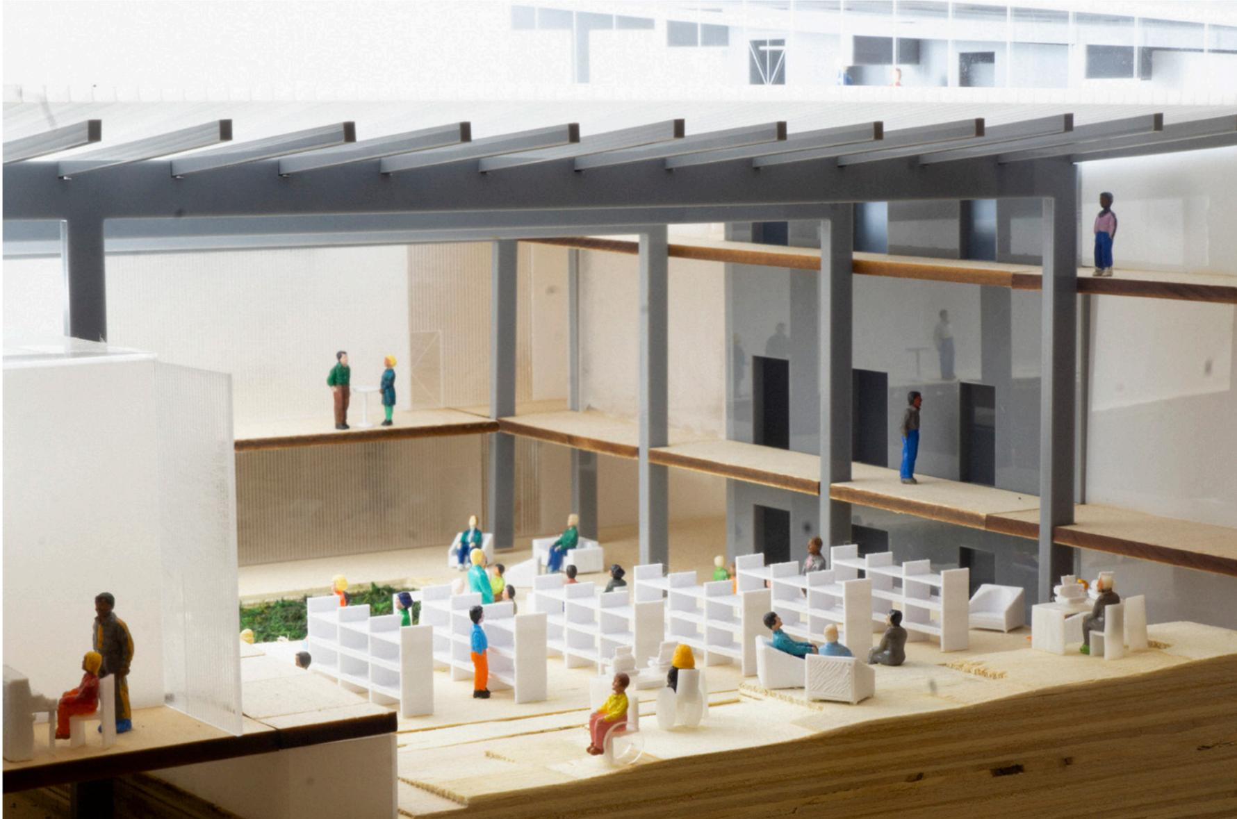
▲ 3/16" sectional model cut through central circulation ramp. ¶ ◀ Circulation & program diagrams. Ramped circulation is prioritized throughout, sidelining stairs. Private programs populate the perimeter of the plan, creating a grand reading room.
