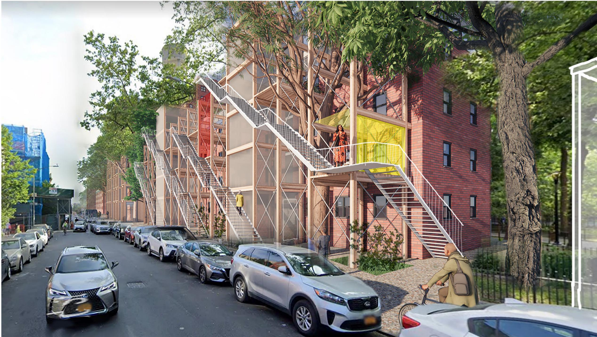
▲ Looking South on Bond St; proposed extension on existing four-story NYCHA building. ¶ Elevators are added outside of existing circulation cores to increase accessibility. Exterior stairs connect intermittent unit extensions, creating secondary access and community stoops.
