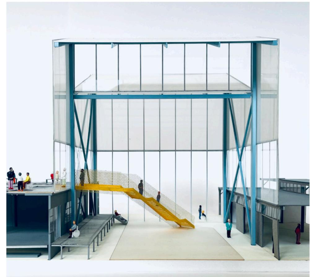
▲ 3/16" sectional model showing new sawtooth structure connecting the existing warehouse buildings.
