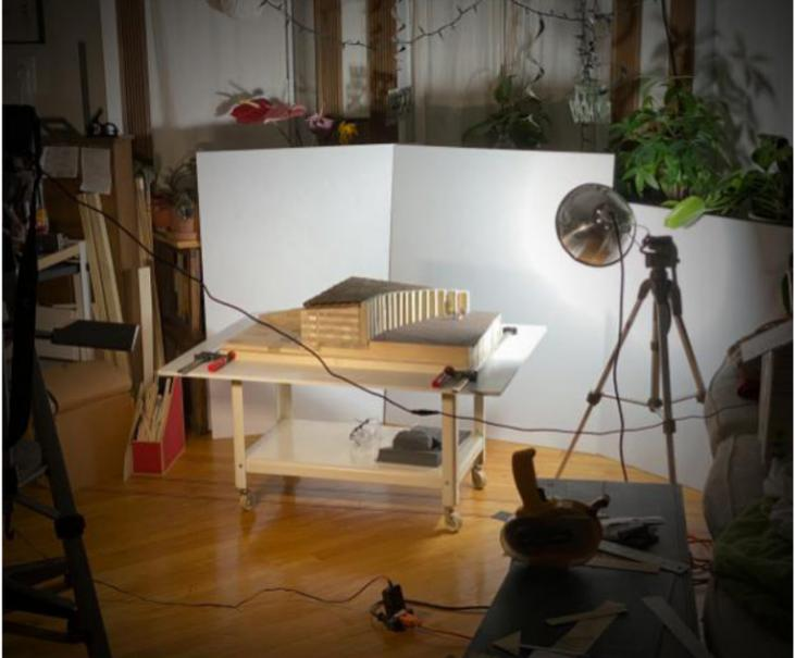
▲ 3/16” model made from hundreds of individual wood pieces. ¶ ▶ Process shot. ¶ Stacked stone walls define voids within the cairn that become the interior spaces for the museum and support program. Timber cleared from the site is reused to form deep glulam beams. The beams span between stone walls in a rationalized 2-d ruled surface.
