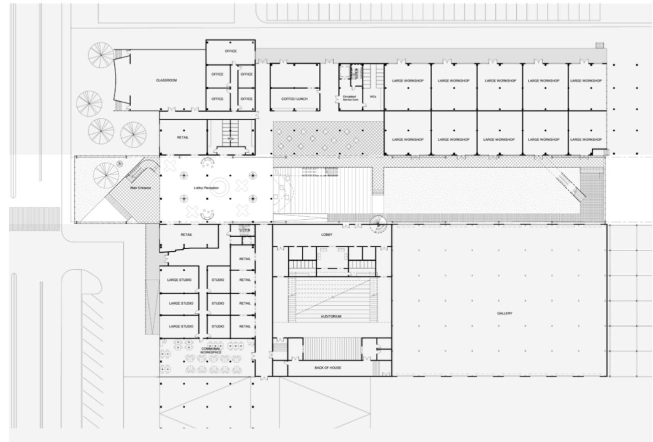
▲ 1:250 conceptual model, top view. ¶ ▶ Ground floor plan. ¶ The incubator program is concentrated in the SW corner of the site. Working with this remaining mosaic of bottling plant buildings, we introduce a new sawtooth shed to unite the incubator as a 'difficult whole.'
