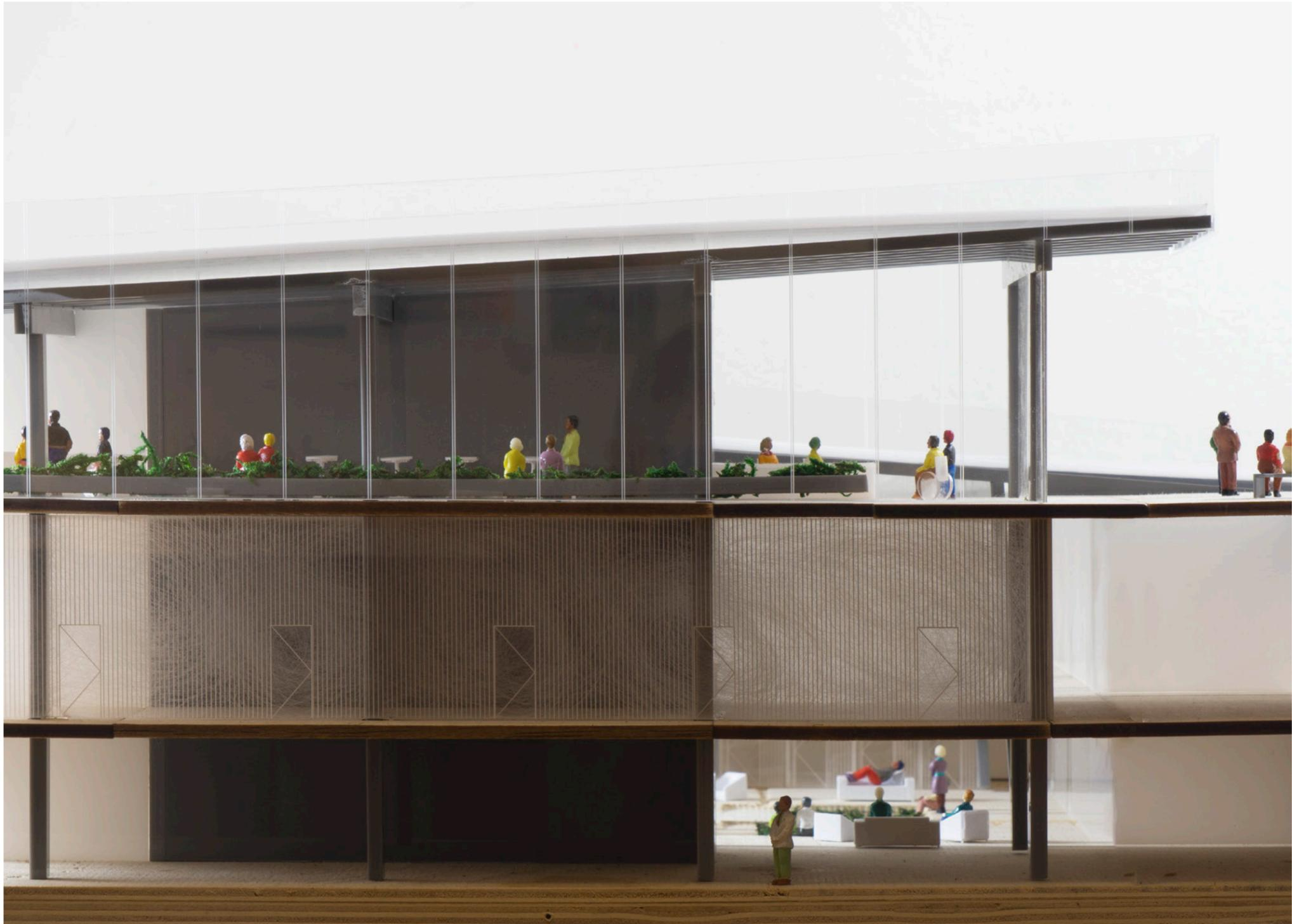
▲ 3/16" sectional model cut along side axis. ¶ Ground floor entry and cafe shown above underground counseling rooms and offices. Terraced stacks terminate two levels below ground in a reading area, lit from above by pavement lights in the occupiable roof.
