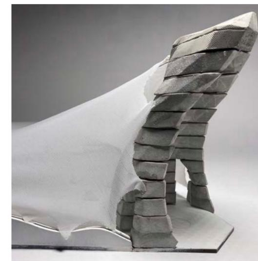
Rockite and fabric models showing the interplay of compression structures with counterbalanced tensile members.
