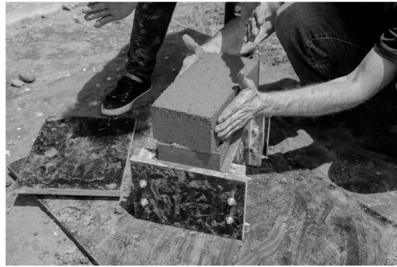
Building local expertise in making the 'permanent' material bricks from local soil
