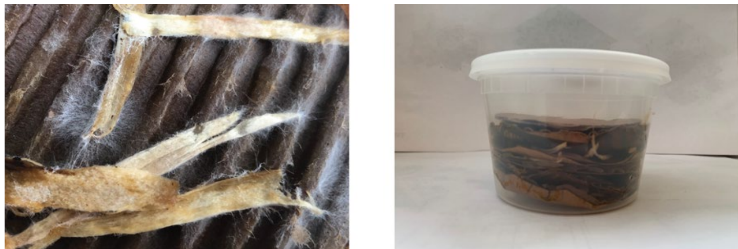
Stage 3 - Leaving the container in a dark environment until mycelium grows from the fibers
