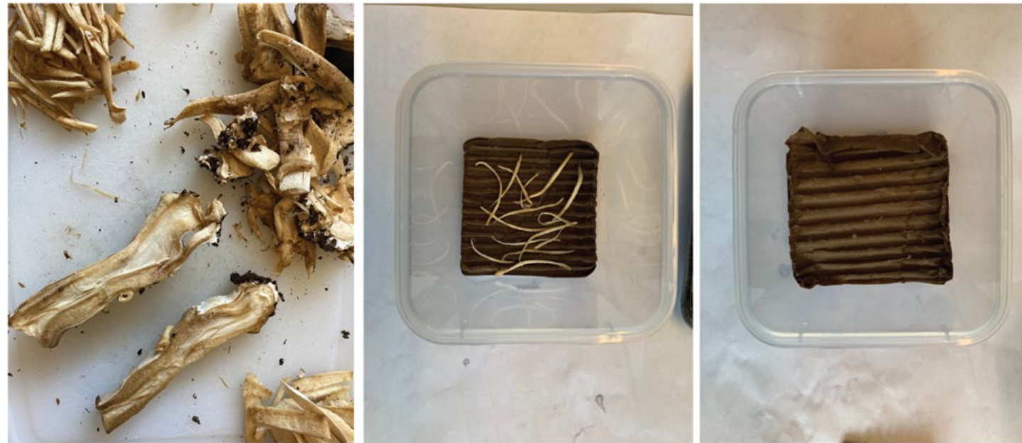
Stage 2 - Stripping the fibers from the mushrooms and then layered them in a container with sheets of corrugated cardboard inbetween
