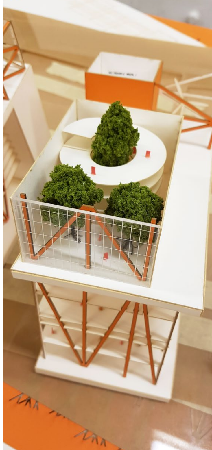
Thanks to the massive truss structures vertically embracing the entire skyscraper, main office volumes can have column-less spaces and create large office spaces for the new type of companies occupying this skyscraper. The main core inside the 'servant' building taking charge of mechanical and structural functions supports the truss structure and the whole building. The spaces inside the main volumes function as office space and also the connection between the servant and the served building.
